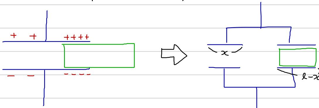
$$\therefore C_{\text{left}} = \frac{\epsilon_0 \omega}{d} x, \quad C_{\text{right}} = \epsilon_r \cdot \frac{\epsilon_0 \omega}{d} (l-x)$$
