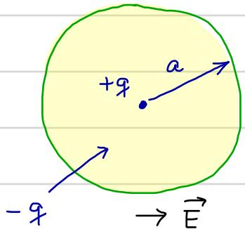
: consists of a point nucleus ( $+q$ ) surrounded by a uniformly charged spherical cloud ( $-q$ ) of radius  $a$ .
