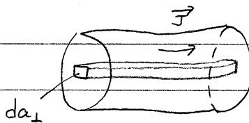
$$\vec{J} = \frac{dI}{dA_L} \quad : \quad \vec{J} \text{ is the current per unit area}$$
