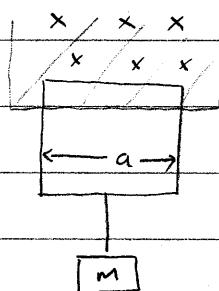
For what current  $I$  in the loop the magnetic force upward balance gravitational force?
