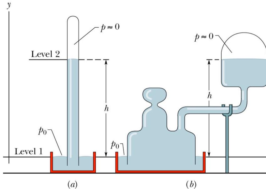
Mercury barometer: a device used to measure the pressure of the atmosphere
