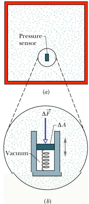
A fluid-filled vessel containing a small pressure sensor
