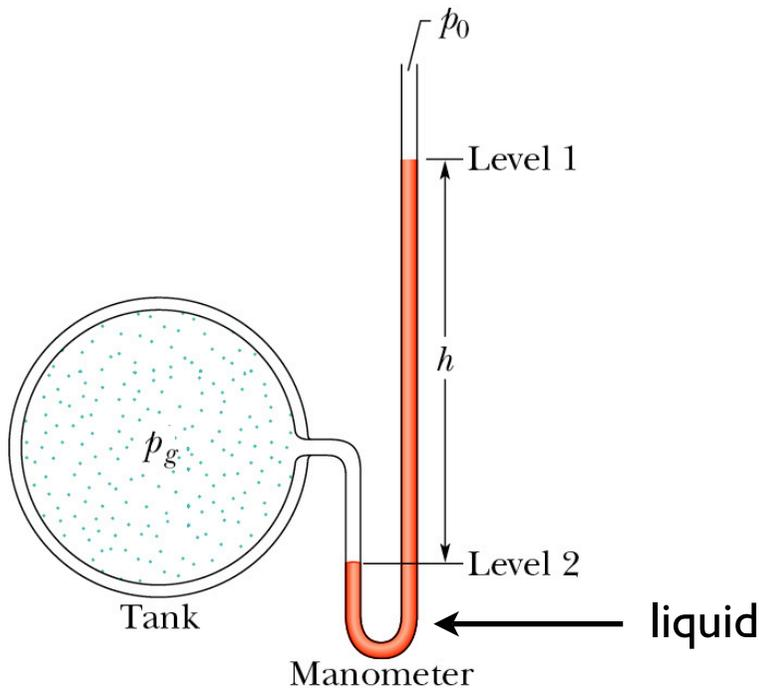
Open-Tube Manometer: measures the gauge pressure of a gas
